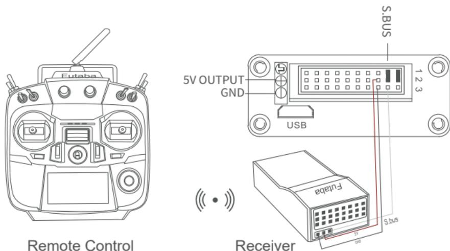
Wiring Diagram Standard Version
