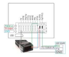
S bus/Rx: connect to Rx2 for track function
