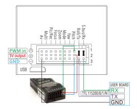
S.bus/Rx: connect to Rx2 for track function.
